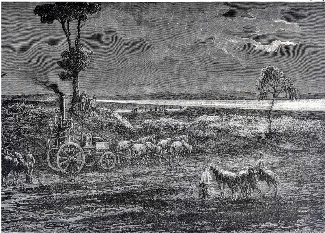
A military reconnaissance with the use of an electric light, illuminating the field, and powered by a steam engine mounted on a horse-drawn carriage.
